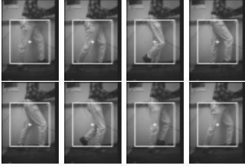
Figure 5: Example training images showing one complete walking cycle. The white box indicates the region of the image used for training.
